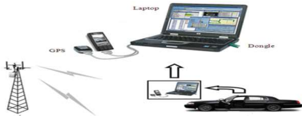
Figure 3: Drive Test kits and illustration [4]
