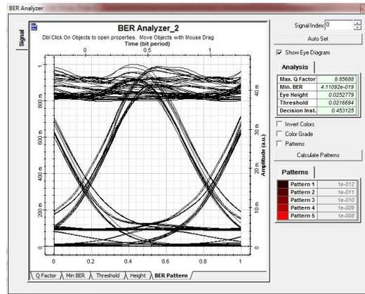
Figure 19: Channel 1 Eye Diagram
