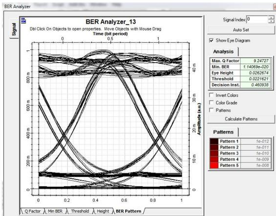
Figure 11: Channel 1 Eye Diagram
