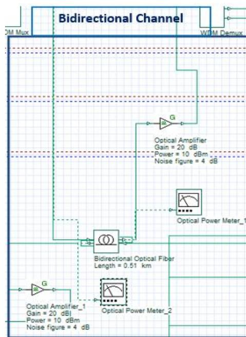
Figure 9: Bidirectional channel of the PON
