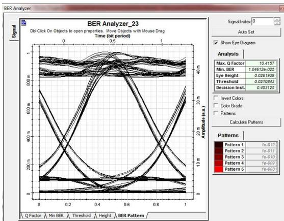
Figure 18: Channel 8 Eye Diagram
