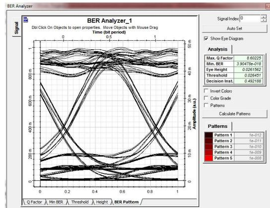
Figure 20: Channel 2 Eye Diagram
