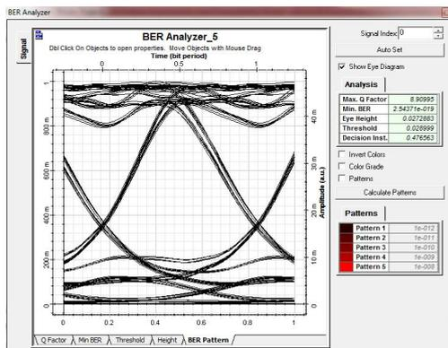
Figure 23: Channel 5 Eye Diagram
