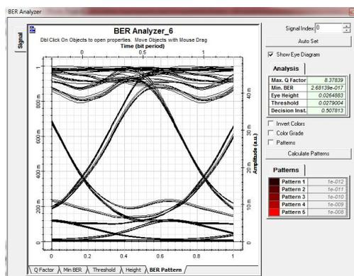
Figure 24: Channel 6 Eye Diagram
