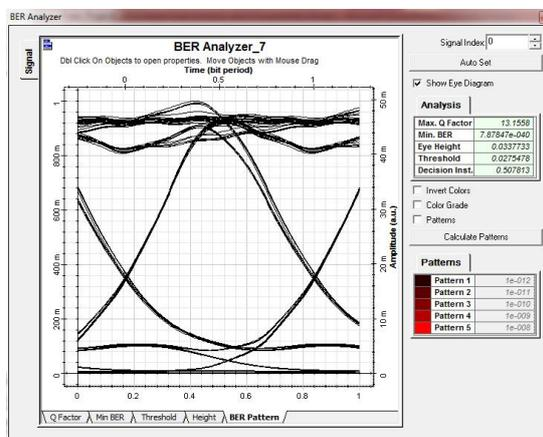
Figure 26: Channel 8 Eye Diagram
