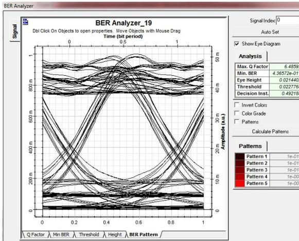
Figure 16: Channel 6 Eye Diagram
