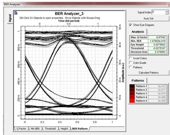
Figure 21: Channel 3 Eye Diagram
