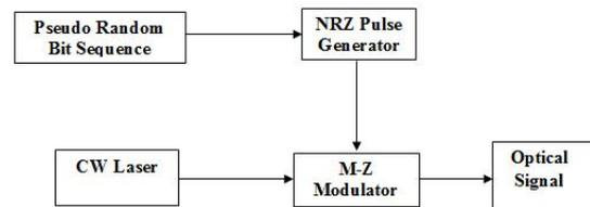
Fig 5: Network Block diagram of Transmitter section
