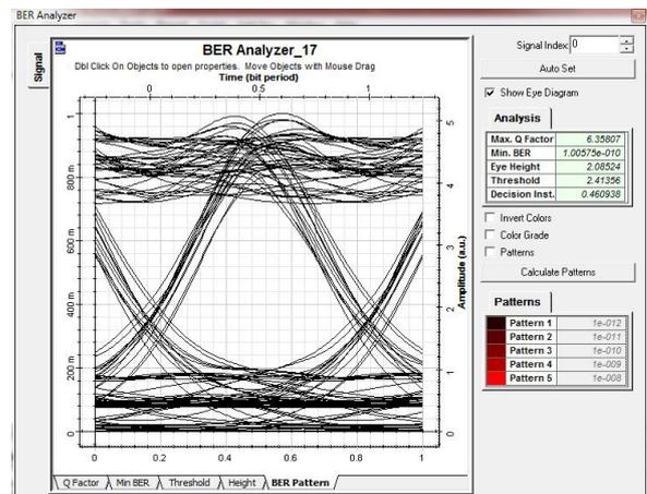
Figure 15: Channel 5 Eye Diagram
