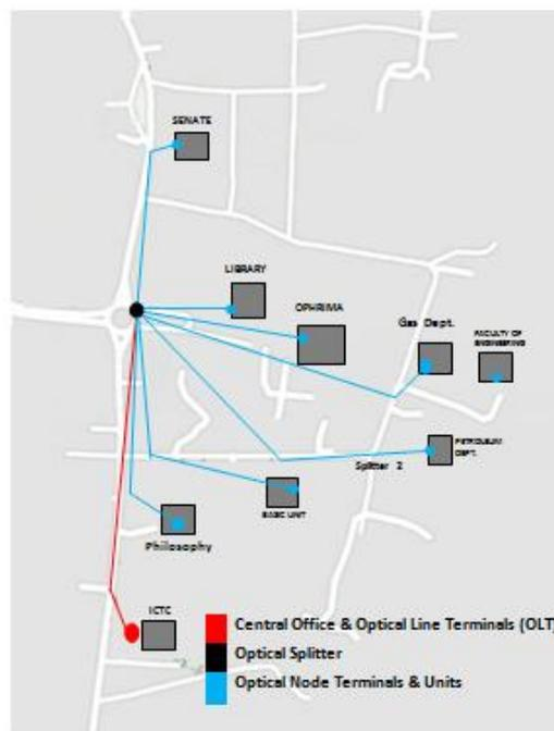
**Fig 3: FTTB layout for the specified network location.**
