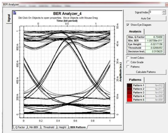
Figure 22: Channel 4 Eye Diagram
