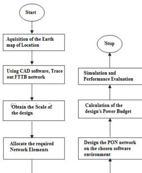
Fig 1: Methodology Flowchart algorithm
