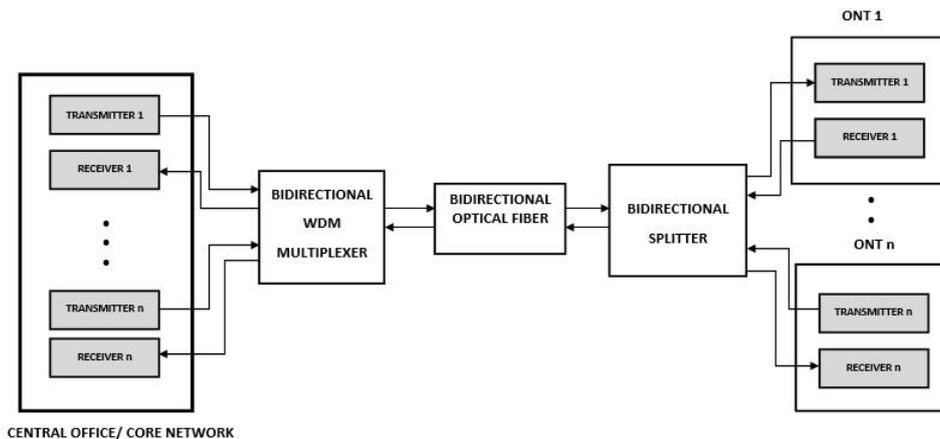
Fig 4: General block diagram for bidirectional PON
