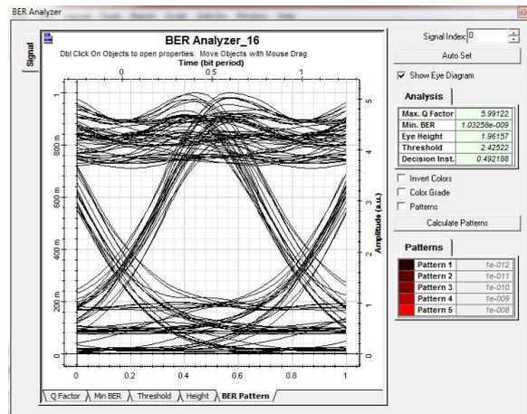
Figure 14: Channel 4 Eye Diagram
