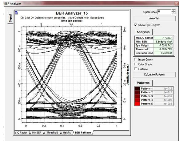
Figure 13: Channel 3 Eye Diagram
