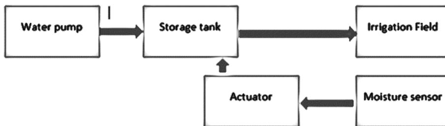
Figure 3.2. Automatic Irrigation Module Block Diagram
