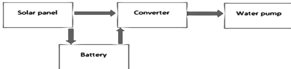
Figure 3.1. Solar Pumping Module Block Diagram
